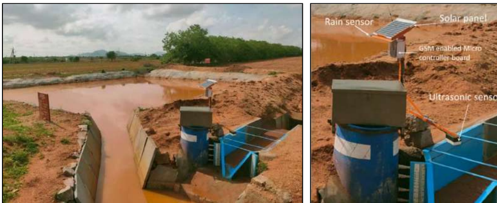
Runoff gauging equipment installed at field & Different components of gauging equipment
